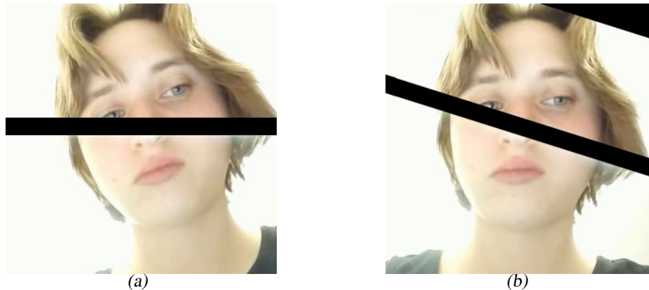
Figure 6.7.: Face alignment. (a) Input frame. (b) Rotated frame to have the eyes horizontally aligned.
